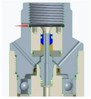
2. Pull out the cartridge kit with M4 screws
